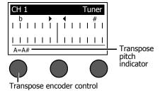
Press the **Transpose** encoder control to select the transpose mode.
