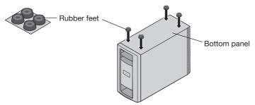
Vibration can cause speakers to move, particularly if placed on a smooth surface like glass or highly polished wood. If you are placing the center speaker on such a surface, you can attach the included rubber feet to the bottom of the speaker for greater stability.
