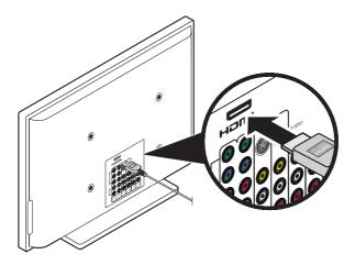
**C.** Insert the other end of the HDMI cable into the **HDMI OUT Video to TV** connector on the control console.
