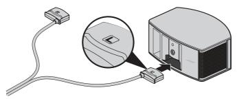
D. Insert the R plug into the right (R) speaker.
