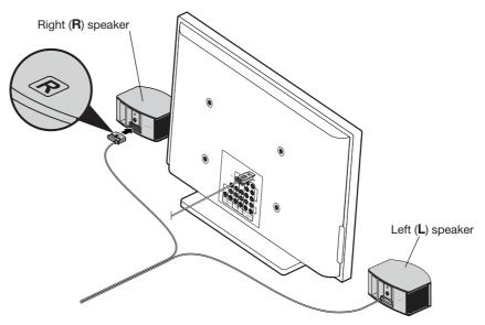
E. Insert the free end of the speaker cable into the SPEAKERS connector on the Acoustimass<sup>®</sup> module.
