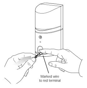
**CAUTION:** Do not connect your amplifier or receiver directly to the cube arrays. Cube arrays must be connected directly to the Acoustimass module or damage will result.
